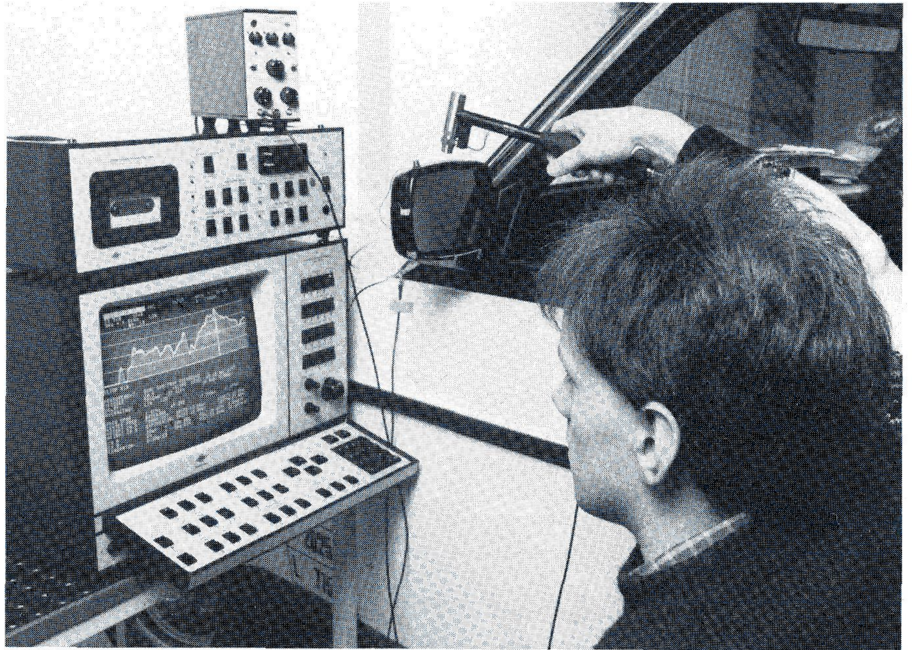
Brüel & Kjær supplies a wide range of equipment for modal testing. The many different applications of modal testing include trouble-shooting noise and vibration problems, design optimization, structural monitoring, and the verification of analytical models of structures
